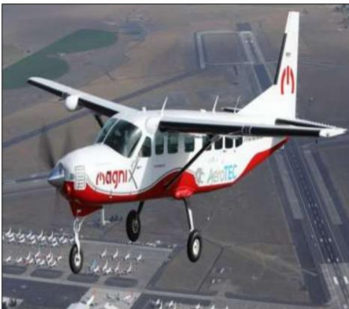
Pictured: The modified Cessna Caravan that had its first flight at Moses Lake, powered by electric batteries. Source: MagniX Twitter page.
